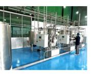
Planet's Pick is in operation since 2016 and is the only producer of extra live coconut oil from Sri Lanka, which uses an outstanding centrifugal process to separate the oil from fresh coconut milk, to derive at a unique superior virgin coconut oil.
